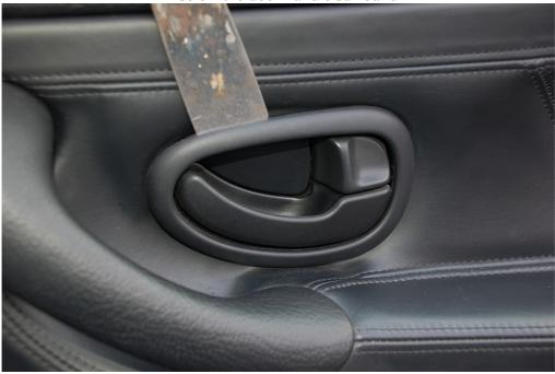
prise out the stopper in the centre of the door and unscrew the bolt inside securing the bottom of the door pull handle to the door. I requires a T20 torx piece. It is a bit awkward to locate the screw driver in the screw as it's up at a 45 deg angle.
