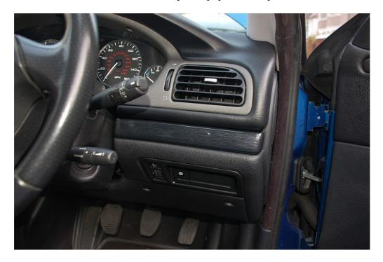
The glove box trim is removed by undoing the 5 screws (torx 20 I think, may be 15) in the inside of the glove box. Just screw the new trim on in its place
