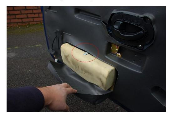
Release the rod that connects the door handle to the door lock. This can be done by looking behind the door handle from the top. Just pull the rod towards you (away from the door) against the spring and it should drop down.
