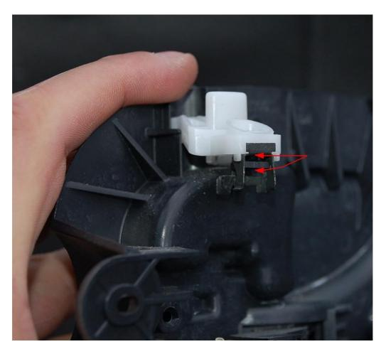
Slip the door opening rod into the hole on the back of the new handle and position against the door. I used some machine bolts and nuts with some washers to secure the new handle on
