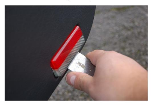
Prise out the electric window and wing mirror controller. I found placing the spatula nearer to the bottom worked best.
