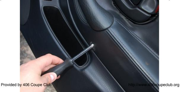
Now remove the screw holding the top end of the door pull handle to the door with the T20 screw driver
