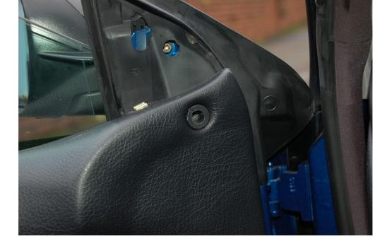
To take the door card off start pulling it away at the bottom and up the sides. once it is loose it should just lift up and unhook from the door. If the card has never been taken off before it will take a bit of effort to release and there will be lots of horrible snapping sounds. This is just the plastic pins that hold the card on coming out.
