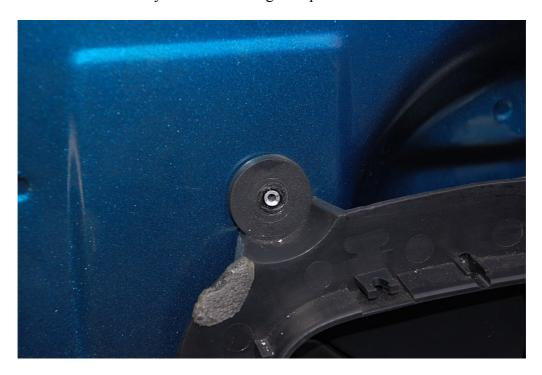
Once all the rivets are off, pull the whole handle mechanism outwards a little and tilt it down at the front to let the rod for the door opening mechanism slide out.
